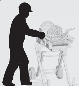
Proper location of the operator while operating the machine.
