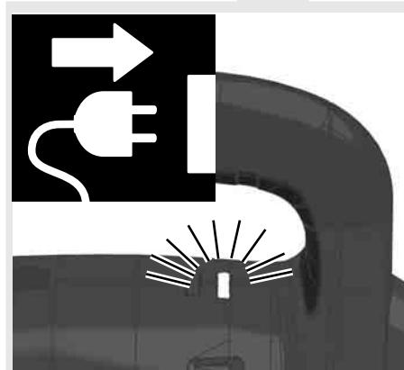
The control lamp flashes: The restart cut-out is active.
